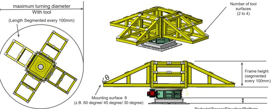
Pedestal/Spacer/Elevation/Platform (segmented every100mm)
